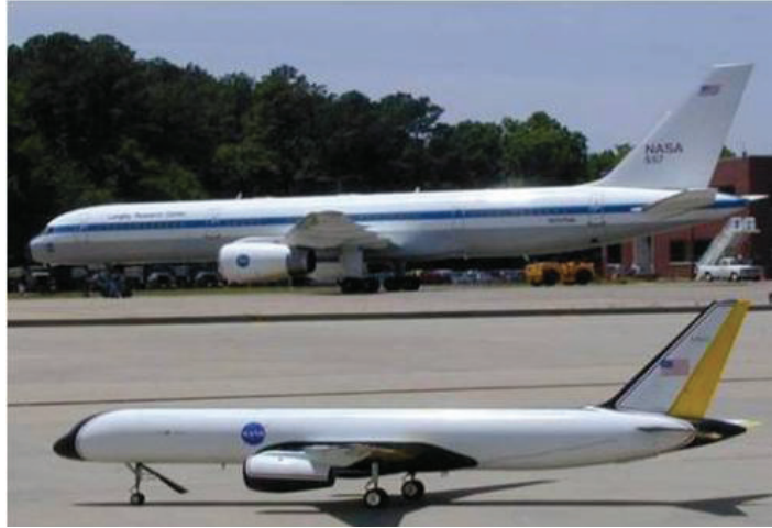
Figure 1: Boeing 757 and GTM Remotely Piloted Vehicle at NASA Langley Research Center
