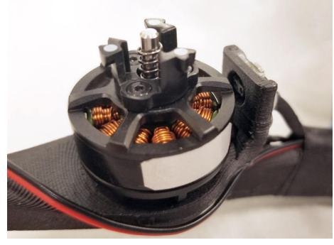
Fig. 2: Motor (propeller removed) with optical encoder that measures rotation speed. The optical encoder lens, and accompanying reflective strip can be seen to the right, and on the front side of the motor hub, respectively.
