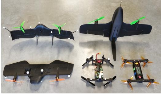
(a) 3D printed vehicles including quad-rotors, tail-sitters
