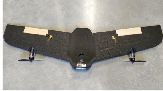
(b) A fixed-wing configuration featuring 3D-printed parts
