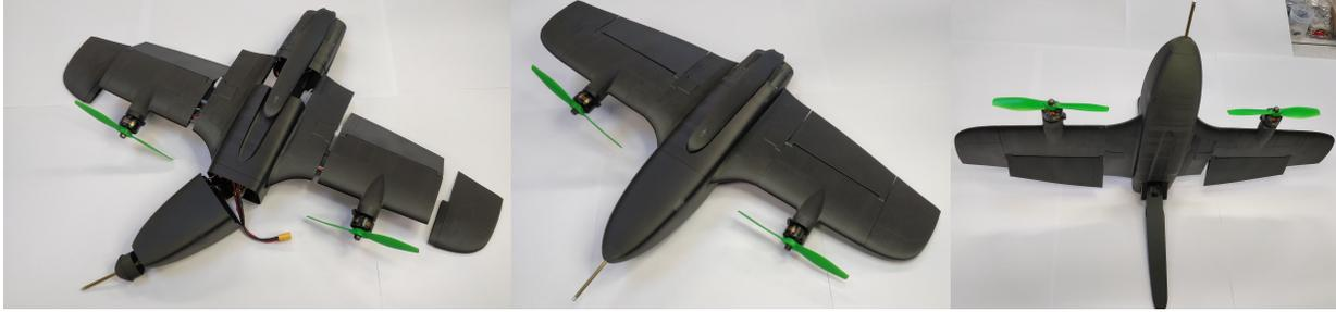
**Fig. 11** Alpha tail-sitter configuration featuring the modular design advantages.
