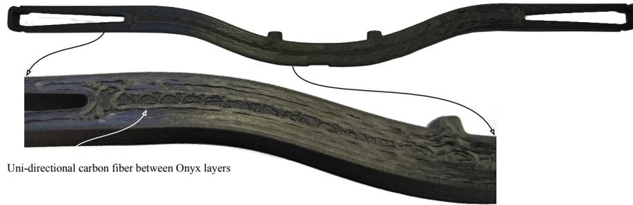
**Fig. 4 3D printed spar structure, shown with inner layer materials.**
